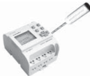
Fig. 2.1 Remove LCD panel as instructed
