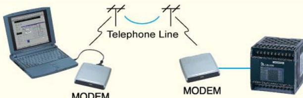
Program and data can be monitored, uploaded or downloaded using the programming tool remotely via MODEMs.
