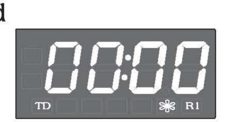
When Relay1 (Heat/Cool) operates, relay2 will operate at the same time. Relay 2 will be "Off" after operating for the set time from the "Off" time of Relay 1. It removes the remaining heat after Heater/cooler stops.
