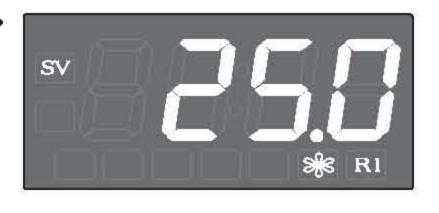
Differential Value is applied to above and below the Selection value. For example, when No.1 selection value is 25.0, No.2 differential value is 1.5, the range of ON/OFF is 23.5~26.5°C. At least, 0.3°C is recommended to protect mechanical system from excessive operation.
